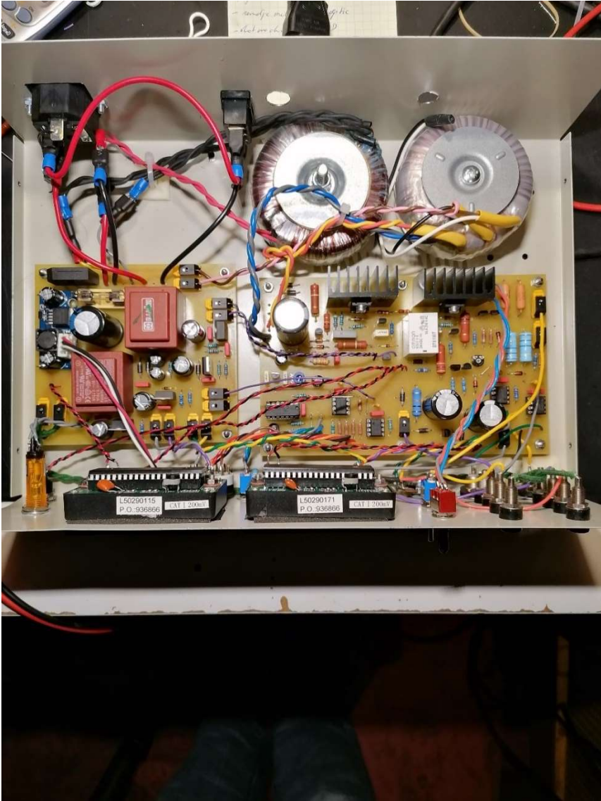
The insides of the mini curve tracer:
